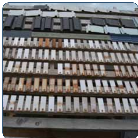
TEST RACK WITH STAINLESS STEEL SAMPLES
